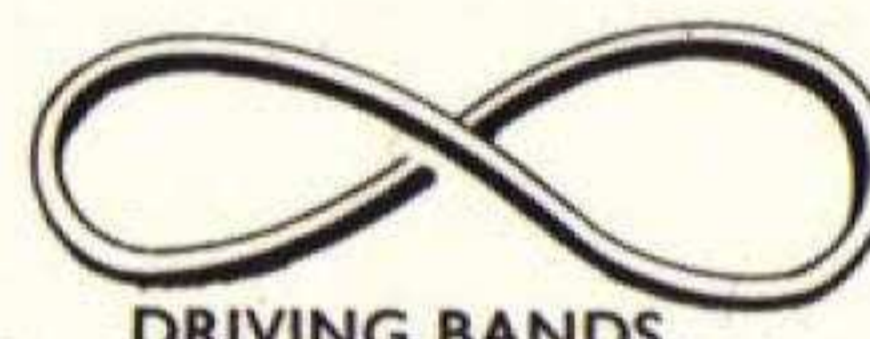
DRIVING BANDS light 186 - 2 1/2"; 6 cm 186c - 10"; 25 cm heavy 186a - 6"; 15 cm 186d - 15"; 37 1/2 cm 186b - 10"; 25 cm 186e - 20"; 50 cm
