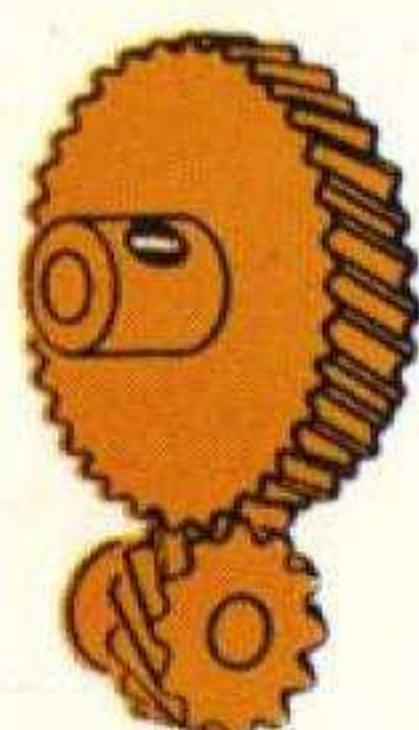
HELICAL GEARS 211a - 1 1/2"; 12 mm 211b - 1 1/2"; 38 mm can only be used together.
