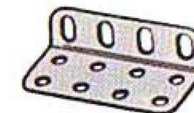
GIRDER BRACKET 161 - 2" x 1" x 1/2"; 50 x 25 x 12 mm
