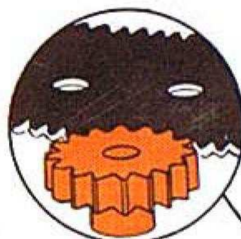
LARGE TOOTHED QUADRANT PINION 167c
