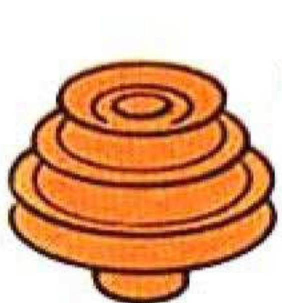
123 - 1½" × 1" × ¾"; 32 × 25 × 19 mm CONE PULLEY
