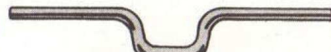
134 - 1"; 25 mm CRANK SHAFT
