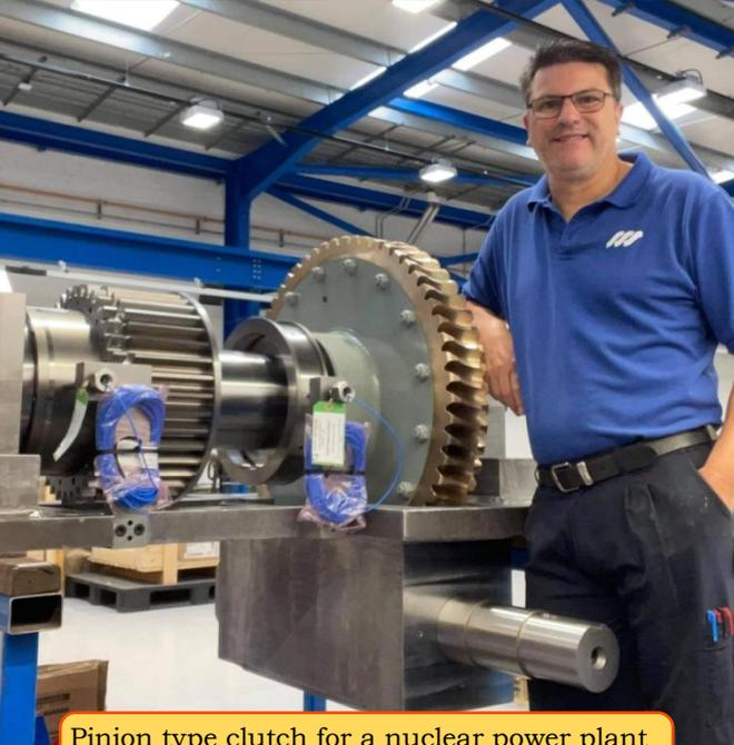
Pinion type clutch for a nuclear power plant currently under construction in the UK
