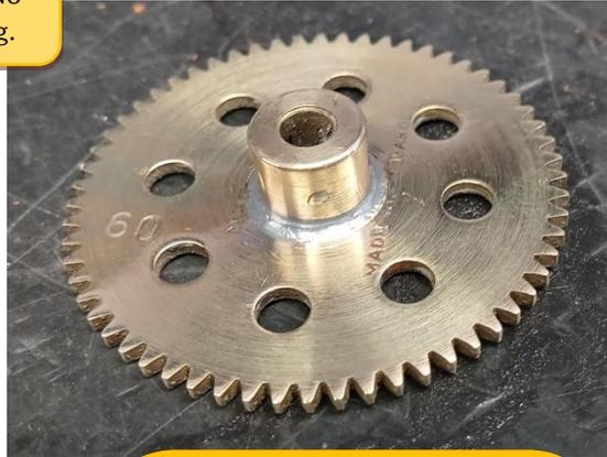
Mick Berg - USA. I found that by using a heat gun, a part can be heated up enough to melt solder. I hadn't thought to try this before. So now I think this must be the most reliable way to fix a loose boss. The excess solder can be trimmed off in a lathe or similar device so it's quite a neat fix. It works on steel or brass. I was glad to be able to fix one of my very valuable 60-tooth gears!
