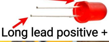
The most common round LEDs on the market are 3mm and 5mm. Any other size is a bit of a rarity. Plastic bezels are easy to find and are cheap as chips. It so happens that the bezel for a 3mm LED is made to snap into a 4mm hole. Perfect for Meccano!
