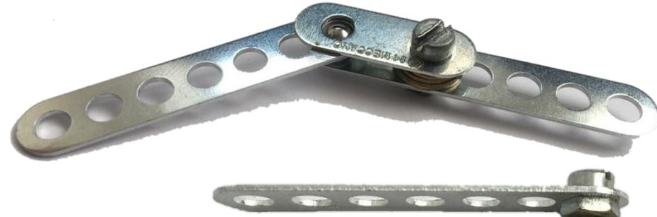
My own no slop pivot joint. A bolt in a threaded hole has less slop than a rod in a plain hole. Richard Payn.
