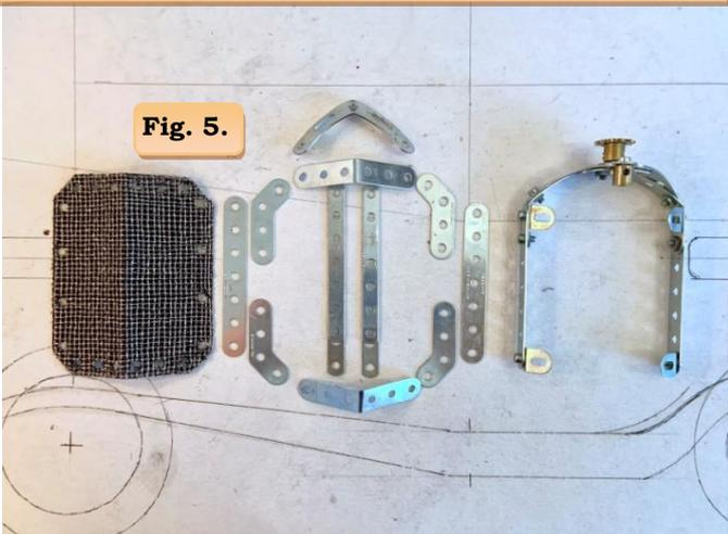
For the radiator grille I made a fabric out of metal threads and polyester that looks as similar as possible to the original. The 133c obtuse Corner Brackets were just right for shaping the radiator. Fig. 5.
