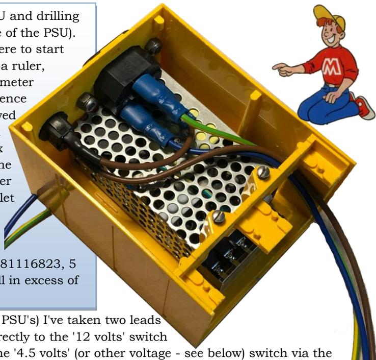
In most cases (I now have 4 of these battery box PSU's) I've taken two leads from the DC +ve and -ve output and fed one directly to the '12 volts' switch and the other to the '4.5 volts' (or other voltage - see below) switch via the buck converter (The buck converter has a screw potentiometer and a digital display for its output voltage). Once wired and tested, the end plate can be glued back into position. This is a little awkward, but everything DOES fit!
