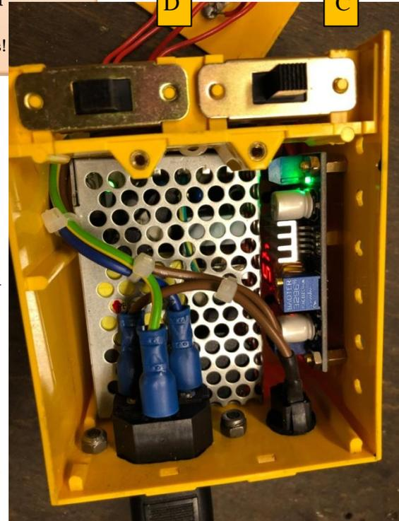
The power supply units themselves are from RS ([www.rs-online.com](http://www.rs-online.com)) and cost around £12-£15. I bought 2 variants, 230vAC to 12vDC @ 2.2A (RS No. 621-0578) and 230vAC to 24vDC @ 1.1A (RS No.621-0584). These are sized perfectly for fitting in the battery boxes.
