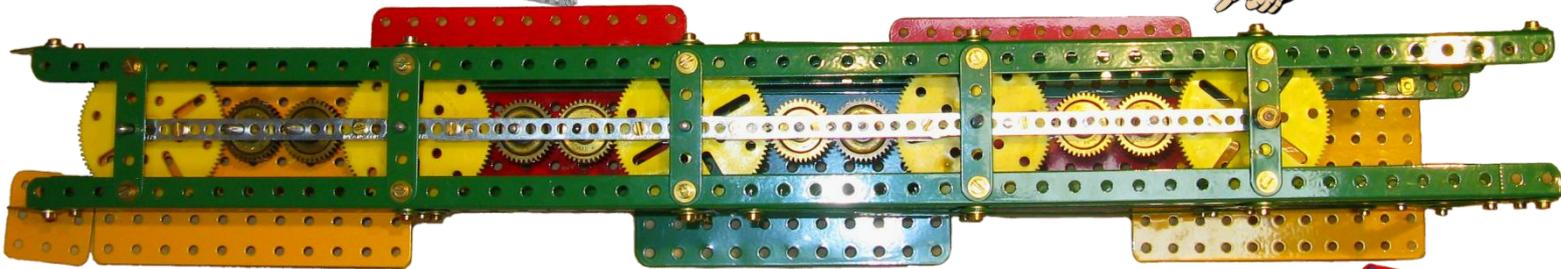
I did run into a problem straight away though, in that as I had insufficient 3 1/2" Gears available to drive the five hexagons I used 2 1/2" Gears instead, with 1" idler Gears in-between instead of the 1/2" Pinions Keith had used. I placed all gearing within the staircase framework rather than below it, and used 1/4"-spaced Narrow Strips to mount the idler Gears, Fig. 3. My hexagons, Fig. 4, are a slavish copy of his.
