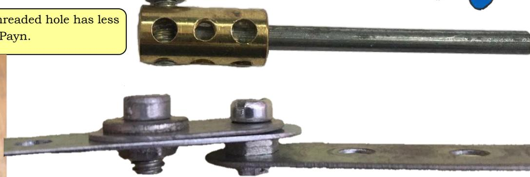
Another easy way of doing a play-free joint. Make the hole smaller by clamping a fishplate over the hole then slide it do the bolt just goes through. Then locknut a strip below. Richard Payn.
