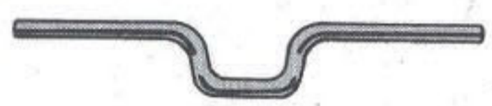
134 - 1"; 25 mm CRANK SHAFT
