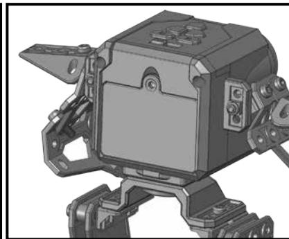
**EN** 1. Open the battery door with a screwdriver.
