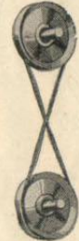
S.M. 17—Method of reversing motion of driven shaft by means of a crossed belt.
