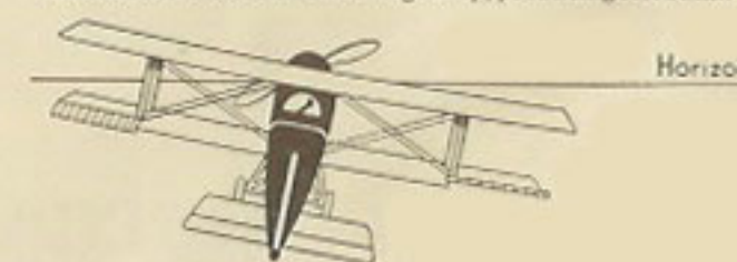
A right bank is brought about by moving the stick to the right.
