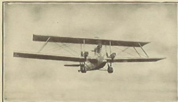
The six-engine Italian Caproni bomber, which is the world's largest bombing machine.
