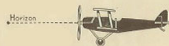
When the control column or "joy-stick" is vertical, the elevator is horizontal, and the machine flies parallel with the ground.
