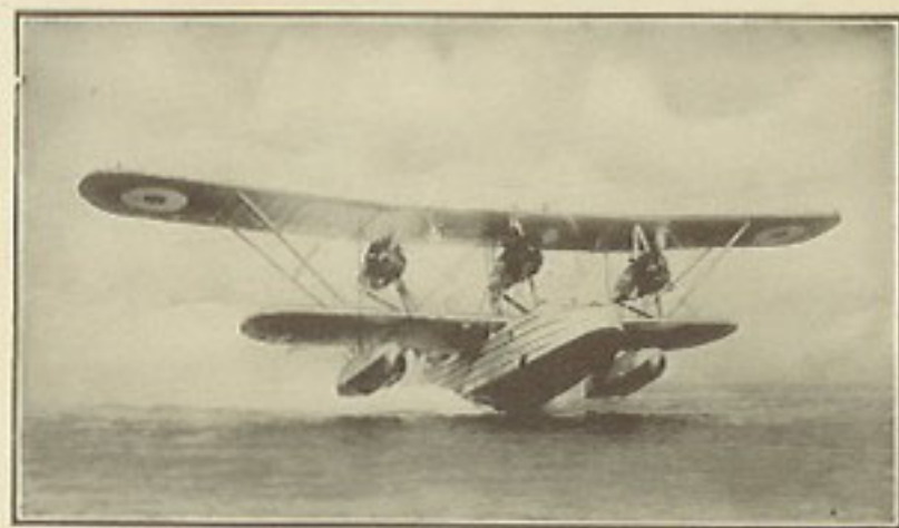
Taking off in the Supermarine "Southampton Mark X," a flying boat fitted with Armstrong Siddeley "Panther" engines.
