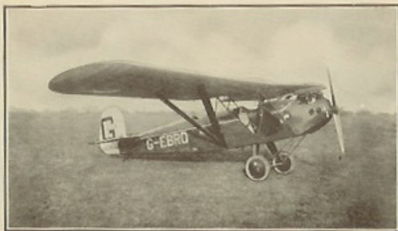
The Westland "Widgeon," a typical parasol monoplane. This machine is a two-seater and is made by the Westland Aircraft Works Ltd.
