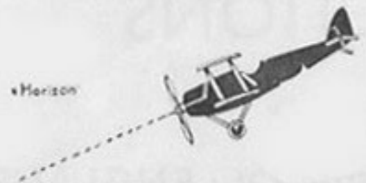
Pushing the stick forward causes the machine to put down its nose and dive.
