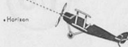
When the stick is pulled back, the elevators are raised and the machine climbs.
