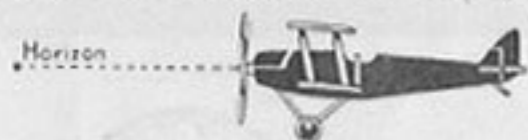
When the control column or "joy-stick" is vertical, the elevators are horizontal, and the machine flies parallel with the ground.
