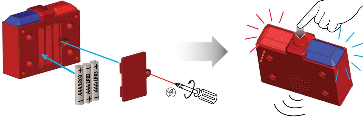
**EN** 1. Open the battery door with a screwdriver.
