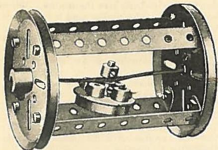
The weight illustrated comprises a Flanged Wheel carrying four Collars, the set-screws of which grip the shank of bolts passed through the Flanged Wheel.
