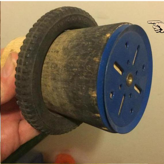
John Ozyer-Key in the UK made this clever device for Richard Payn to use on those difficult hardened tyres that refuse to go onto the pulley.
