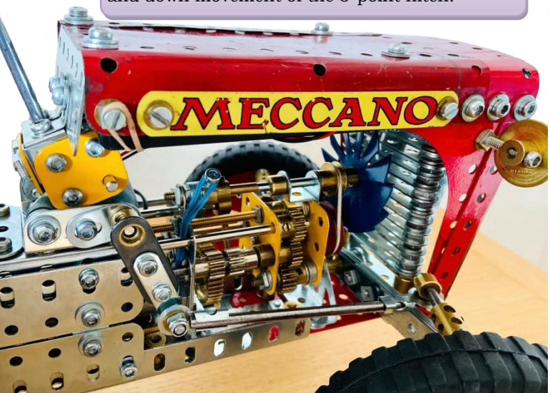
Front transmission cover is still missing. This part of the transmission is responsible for the up and down movement of the 3-point hitch.
