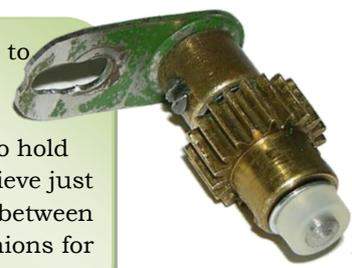
The original model uses a French motor, apparently with a reversing feature. This and the attached gearbox are impossible to decipher from the illustrations or text. So I substituted a Mike Rhoades' 120rpm motor and mounted it where I could on my gearbox frame.
