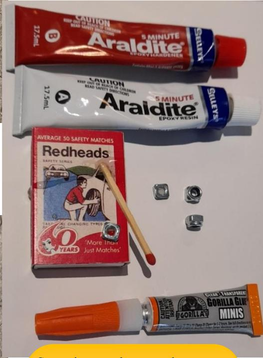
Sometimes nylocs can be too thick. You can turn a standard bolt into a nyloc with a drop of Araldite or any other epoxy resin. Even Gorilla glue seems to work. Just drop in into the hole, let it dry, then run a 3mm drill bit through the hardened glue to help get the bolt started.
