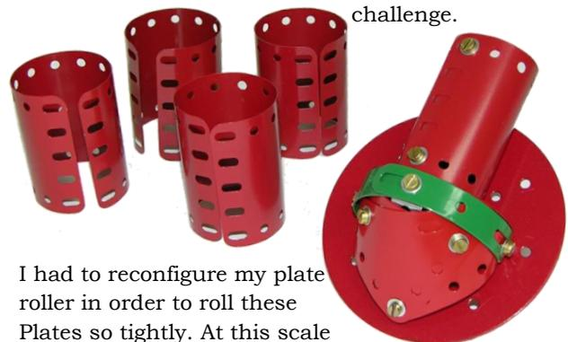
I had to reconfigure my plate roller in order to roll these Plates so tightly. At this scale I needed a nine-hole circumference.
