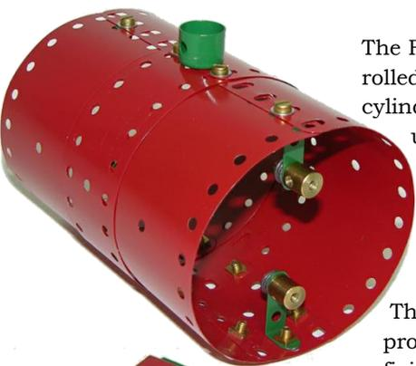
The Flex Plates were rolled to form the cylindrical barrel, using a Flanged Disc, part 168a as the template for the curve. Narrow Angle Brackets and Threaded Bosses provided the Bolt fixing points for the end Discs.
