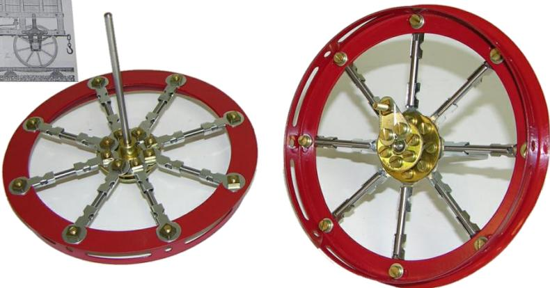
Rather than using Hub Discs for the driving wheels I decided to build-up the spokes on a Circular Girder. Not a great idea. It is very, very difficult to ensure that the Bush Wheel is perfectly centered on the Circular Girder. Maybe Narrow Strips could have been substituted for the spokes?
