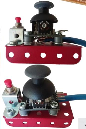
The joystick can be mounted any way you like but I've used a Flanged Plate and 1/4" spaced Narrow Strips to line up with the mounting holes. I chose to solder the 6 wires directly to the PCB rather than use the header pins.
