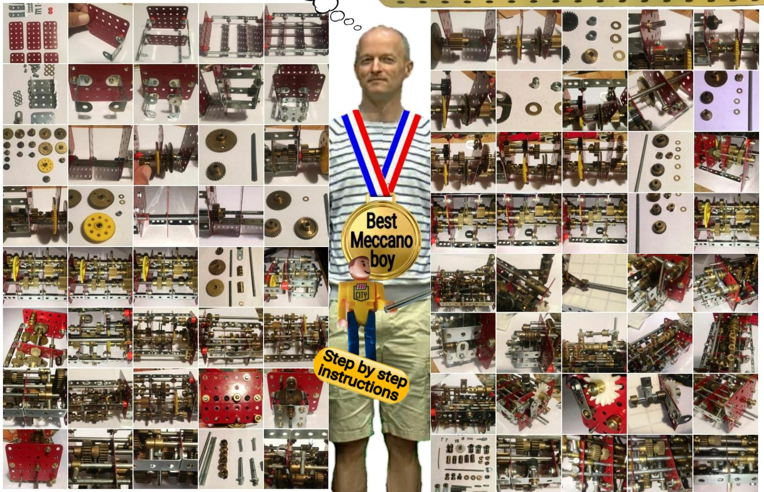
This gearbox gives equally spaced gears that are between 40% and 43% apart, much like a real truck gearbox. The parts required are shown in the photographs along with part numbers and explanations of why some specific parts are used. eg. "The unit will work just as well if the 20t and 56t gears are swapped with 19t and 57t gears."
