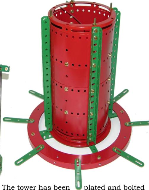
The tower has been plated and bolted to the top Flanged Ring of the roller bearing. The flattened Formed Slotted Strips will connect the roller bearing to the inside of the Sector Plate platform.
